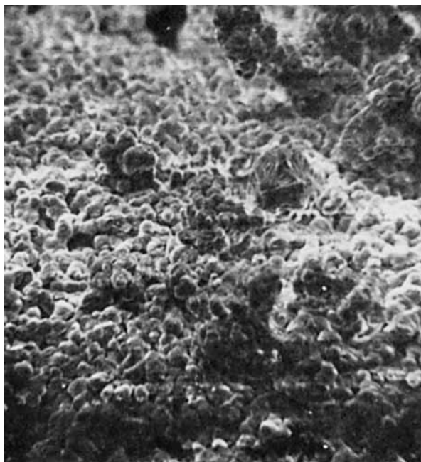
Fig. 1. Typical structure of polyethylene ( \times 1200 ) made with the catalyst. Yield = 1.98 kg/g \text{TiCl}_3 .
